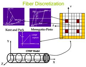
Figure 2 Modeling of FRP-Strengthened RC Girders
